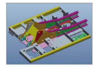
The main beam of the turntable adopts the H-type structure, and the side beam adopts "D-section" structural steel, which has higher overall reliability.
